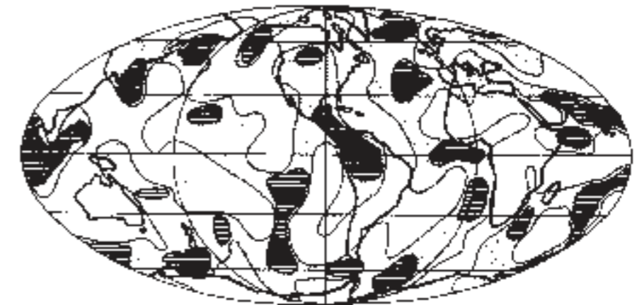
FIG. 4—Isostatic gravity map of earth constructed from spherical harmonic coefficients of degree 6 through 16. Shaded areas are regions of positive anomalies, heavier shaded areas are regions where anomalies are greater than +10 mgal. Note correlations of gravity highs with Iceland, Hawaii, and most other hot-spots (adapted from Kuola, 1970).
